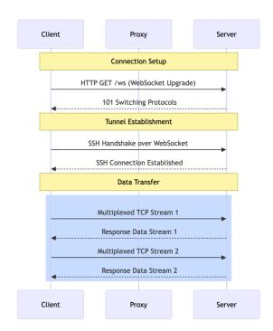
Use Chisel software to Transfer Data Over HTTP tunnel
